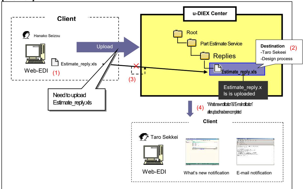
\* This overview indicates the following process: "Hanako Seizou uploads the file 'Estimate\_reply.xls' to the location '/Part Estimate Service/Replies/' at u-DIEX addressed to Taro Sekkei and the Design process".
