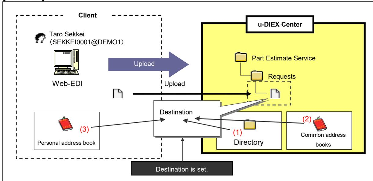
\*This overview indicates the following process: Taro Sekkei sets the destination for data being uploaded.
